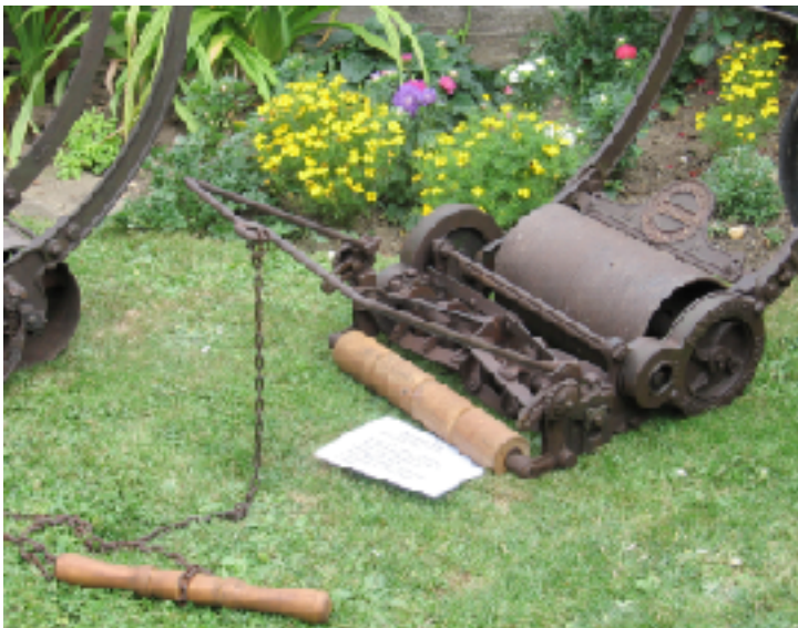
Very early Ransomes mower from collection. The 'husband & wife' version... wife pulling and husband pushing and steering.
